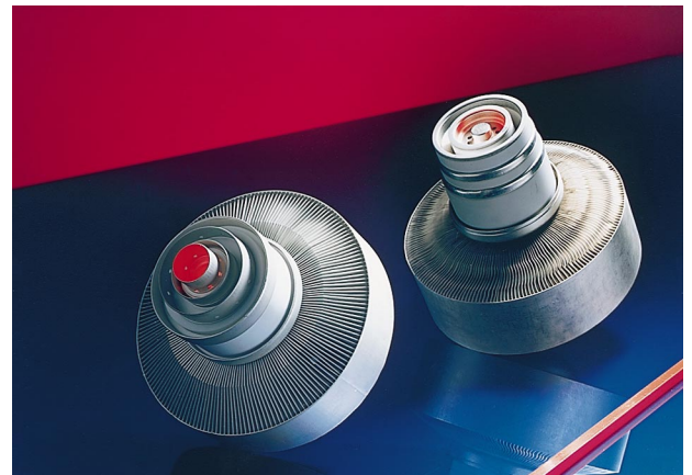
Tubes from different manufacturers may be used: left: RS2068 (Siemens) for 10-kW transmitter right: 4CX20000 (Eimac) for 20-kW transmitter (photo 37915-1)
